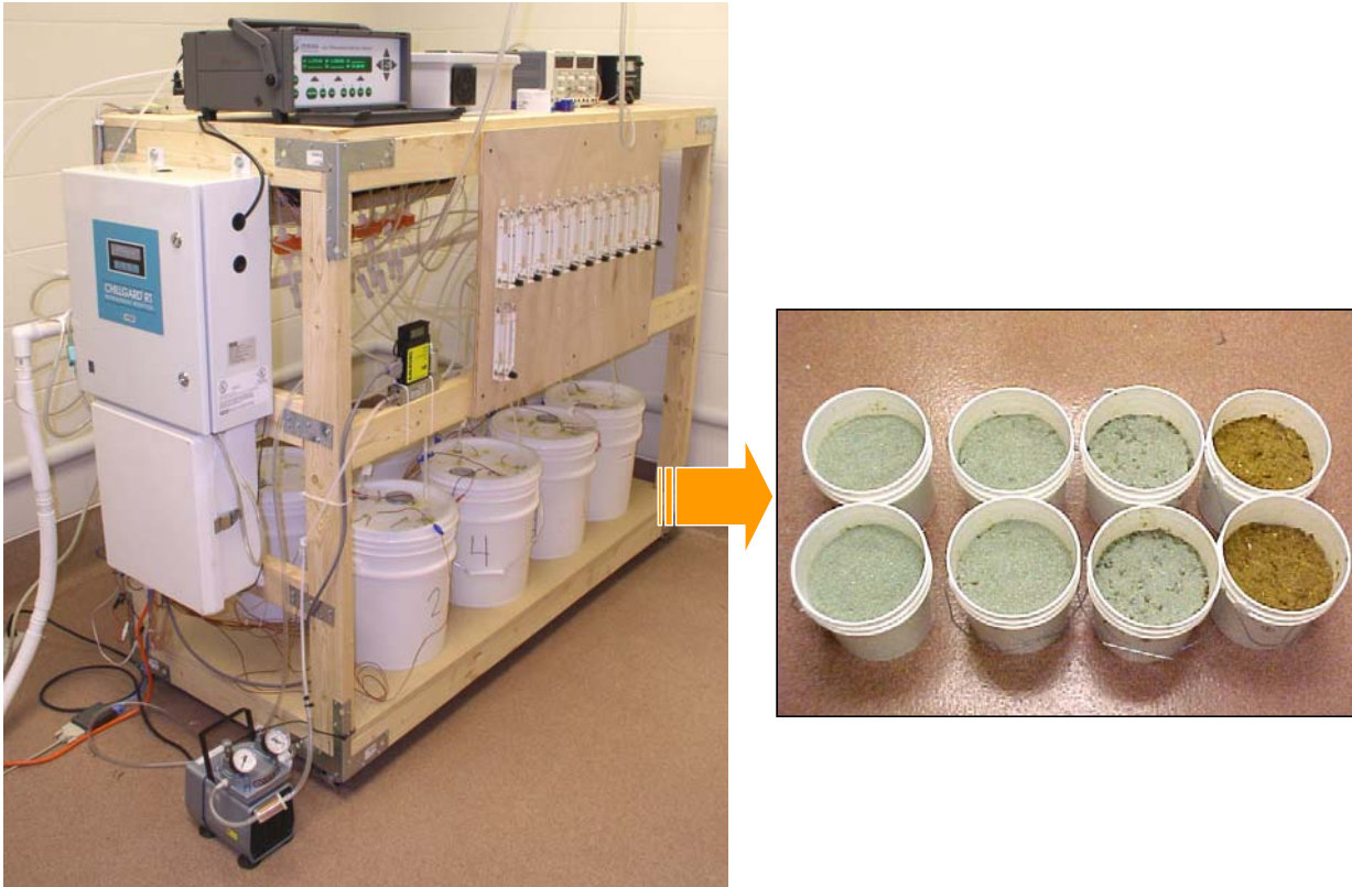
Figure 2b. Photographical views of the lab-scale setup for evaluating efficacy of air emission mitigation strategies. Pictured (right) is topical application of Zeilite on laying hen manure at various dosages.
