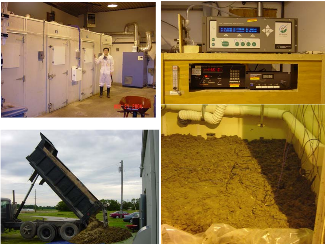
Figure 1b. Photographical views of the air emission chambers and data acquisition system used in our air emission measurement and mitigation studies.
